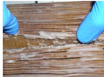
Filters can clog if glycerin levels are too high in the biodiesel used to blend.
